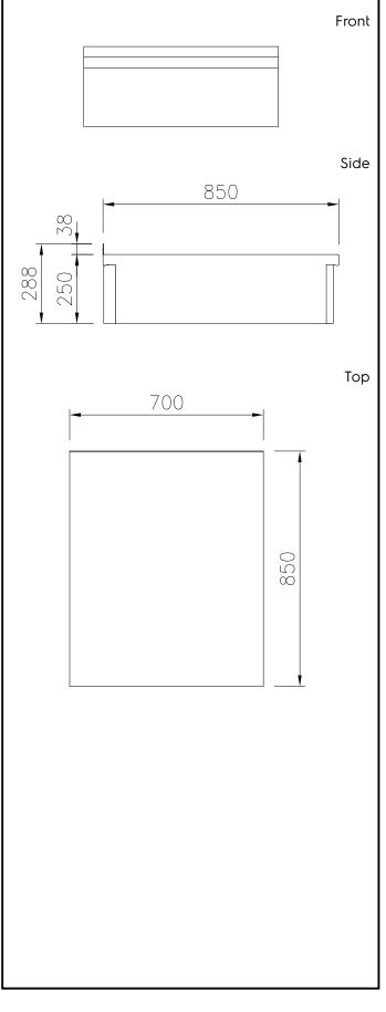
Modular Cooking Range Line thermaline 85 - 700 mm Closed Work top, 1 Side with Backsplash
